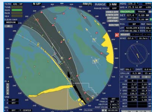
CHART MODE: Radar Display with chart presentation (night, areas filled)
